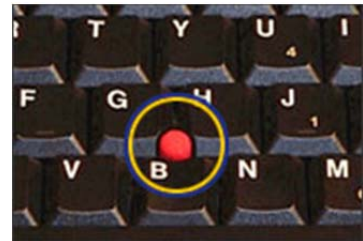
Figure 8 Fingertip joystick for a notebook computer
